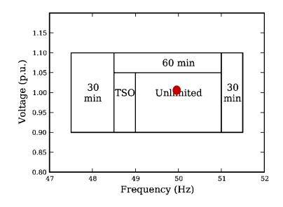
Time before generator is allowed to disconnection during a voltage/frequency deviation
